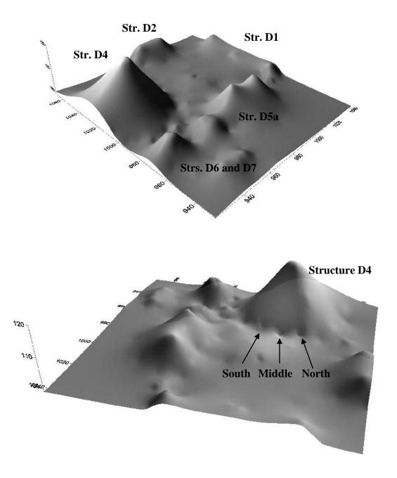
Figure 4.3. Contour map of Group D main plaza produced using a Sokkia Set 530R3 total data station. The top image is on a northeast to southeast axis, and the bottom image is on an east to west axis. The bottom image shows the three large looters' trenches, known as South, Middle, and North, at the base of Structure D4.
